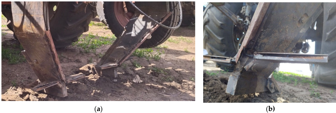
Figure A1. The working organ (a) of the universal deep loosener fertilizer with tillage knives, and a flat fan spraying nozzle (b).
