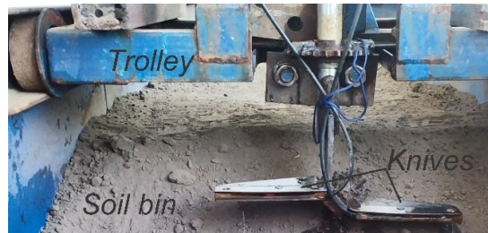
Figure 10. The trolley equipped with knives and sprayers.
